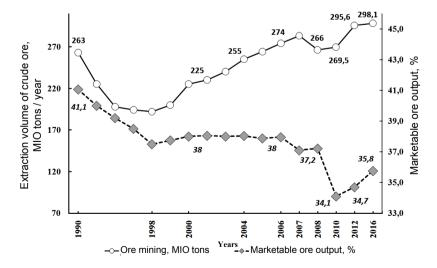
Figure 2. Dynamics of production of raw iron ore and the yield of marketable ore in percentage terms for the Russian Federation for the period 1990–2016.
