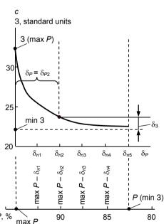
Graphical interpretation of the justification of concessions on the criteria of  $\max P$  and  $\min$  3. a – dependence of criterion P, %, on land use options; b – dependence of the total cost criterion 3, standard units from land use options; c – the dependence between the criteria of total costs of 3 and P.
