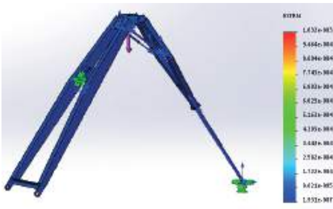
Figure 8. Study of deformations in the support structure of the pipelayer boom.
