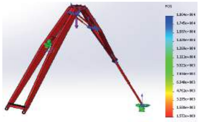
Figure 9. Study of the safety factor in the support structure of the pipelayer boom.
